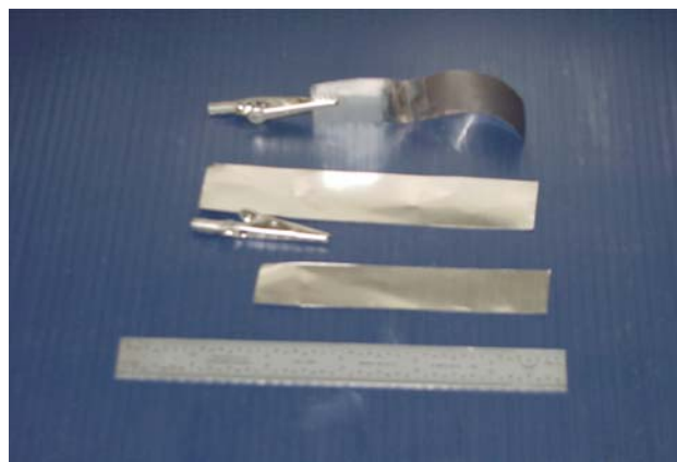
Fig. 1 Macroscopic buckling of AISI 321SS during hydrogen charging
